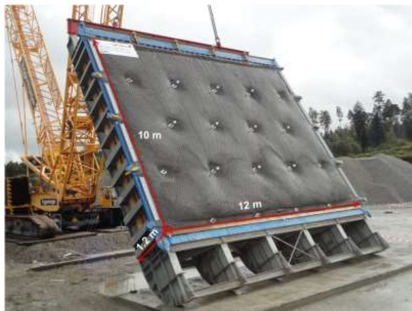
Figure 3. Test setup before the rupture of flexible facing
