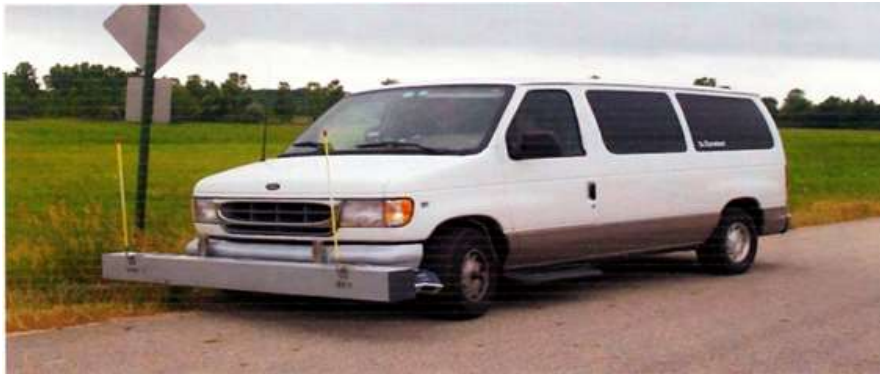
Figure 4. High speed inertial profiler The Dynatest Road Surface Profilometer 5051 Mark II Source: (Own Figure)
