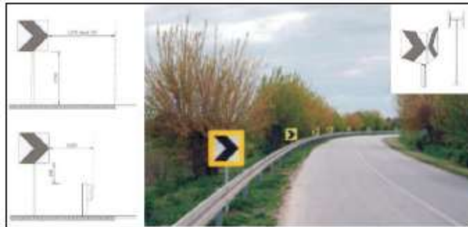
Proper installation of chevrons in curves
