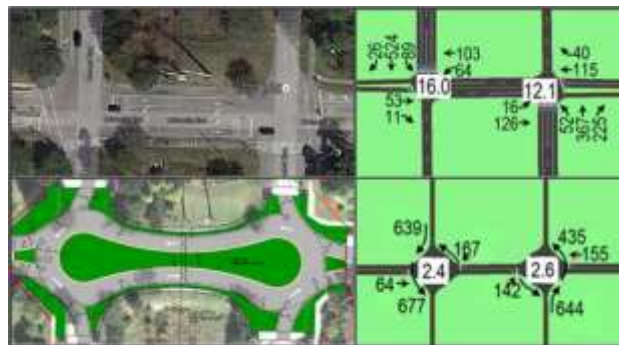
Figure 1. The geometry (left) and volumes (right) for the existing (top) and proposed (bottom) VISSIM model development
