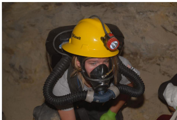
Figure. 2: Modern protection equipment for miners (Source: http://inside.mines.edu/Mining-Edgar-Mine ).
