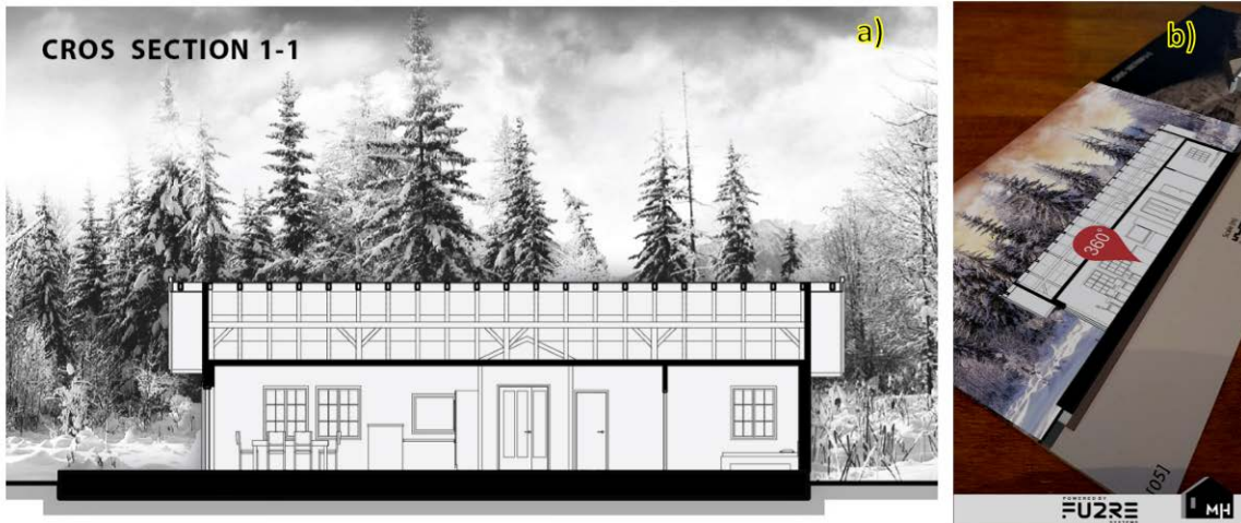
Figure. 7: MH Petra: a) Cross section (marker); b) Augmented Reality presentation of section with 360° button
