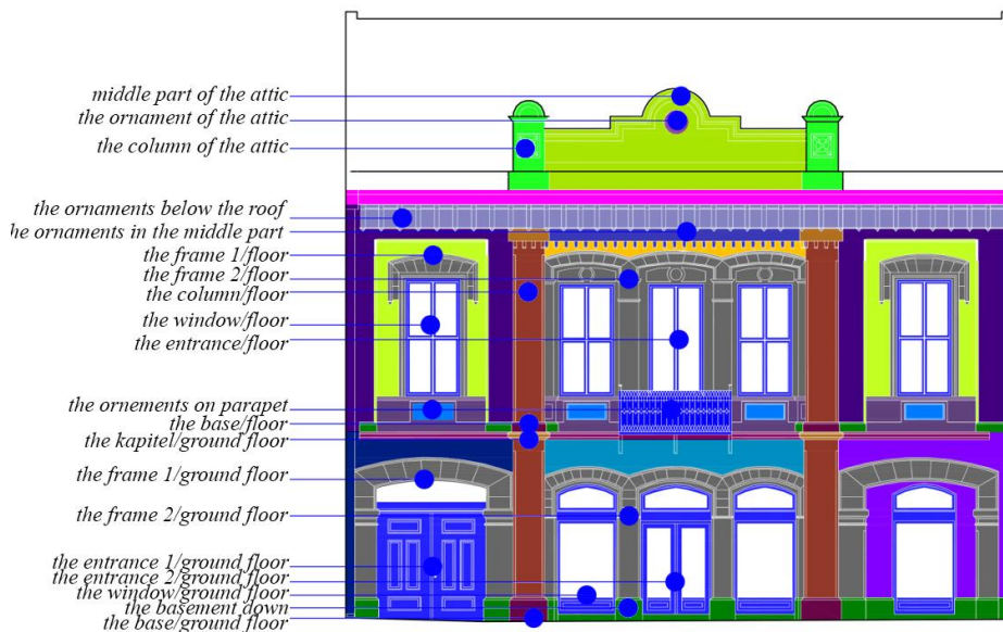
Figure. 3: Example of facade elements belonging to Romanticism (Retrieved from students Marija Mastilović and Boglarka Balint) Analysis of the facades is the basis for the creation of split grammar rules.
