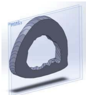
Figure 9: The virtual tibia segment re-constructed in SolidWorks [3,9]
