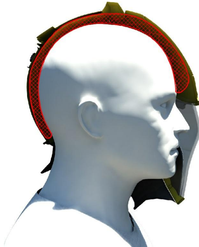
Figure. 17: Head inlay with polyurethane.
