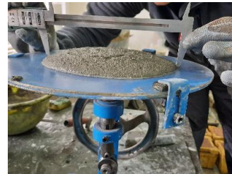
Flow test (at FCE BG)
