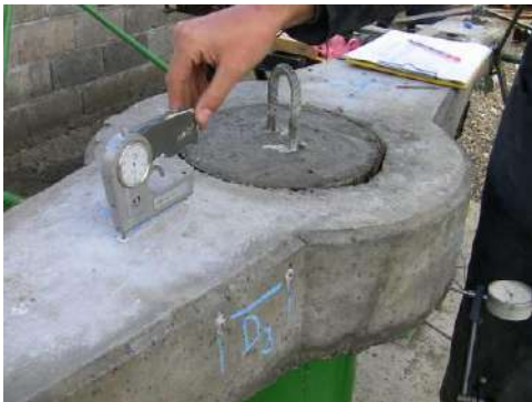
Figure 7 – Measuring of dilatations and cracks
