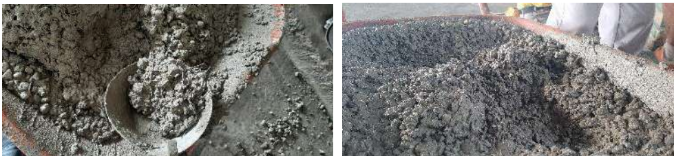
Figure 2 – The appearance of fresh concrete with polypropylene fibers
