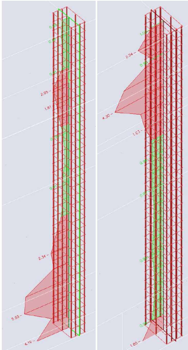
Figure 14 – 2 nd frame south façade column unity checks before and after the urgent strengthening
