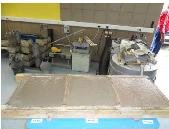
Figure 3 - Repair mortars placed on concrete substrates
