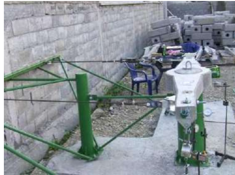
Figure 6 – Experimental setup (testing frame and method of loading of the concrete cantilever)
