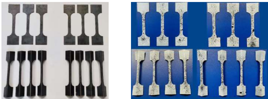
Figure 2 – Coupon specimens before (left) and after (right) preparation
