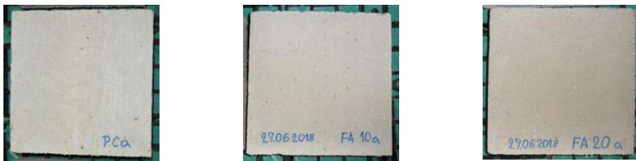
Figure 4 - “Repaired” specimens look after the storage period (mortars prepared with w/b=0.5 ): left – PCa, middle – FA10a, right – FA20a
