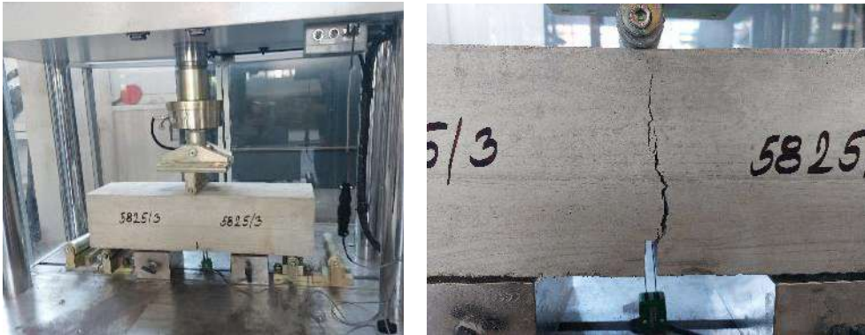
Figure 3 – The position of the beam before the Flexure Tensile Strength according SRPS EN 14651
