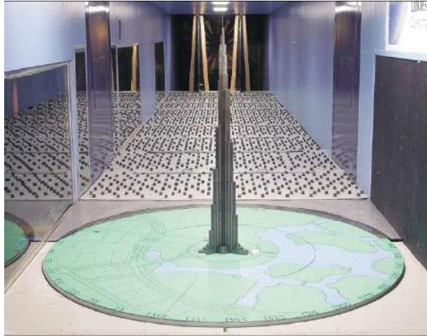
Figure 8 – Burj Khalifa Aeroelastic Wind Tunnel Model (SOM)
