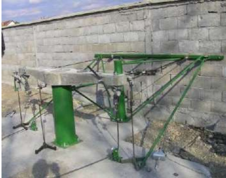
Figure 6 – Experimental setup (testing frame and method of loading of the concrete cantilever)
