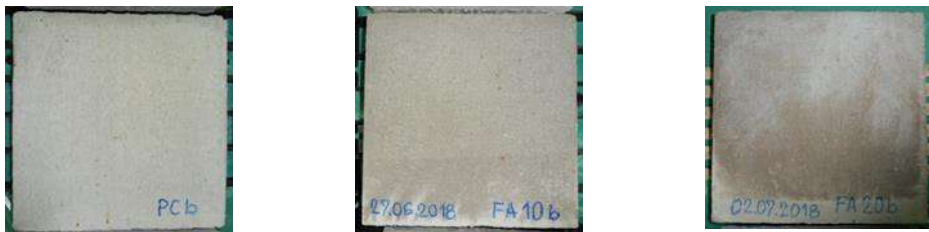
Figure 5 - “Repaired” specimens look after the storage period (mortars prepared with w/b=0.4 ): left – PCb, middle – FA10b, right – FA20b
