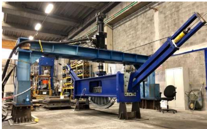
Figure 7 – Fatigue and subsequent friction with ultimate resistance testing
