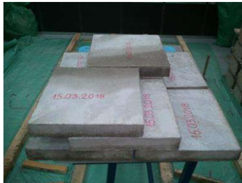
Figure 2 - Reference concrete substrates after demoulding
