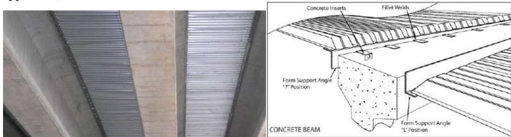
Figure 6 – Left: Stay-in-place forms – view from underneath the bridge (catalog New Millennium Building Systems); right: stay-in-place forms connection detail (catalog LB Foster)
