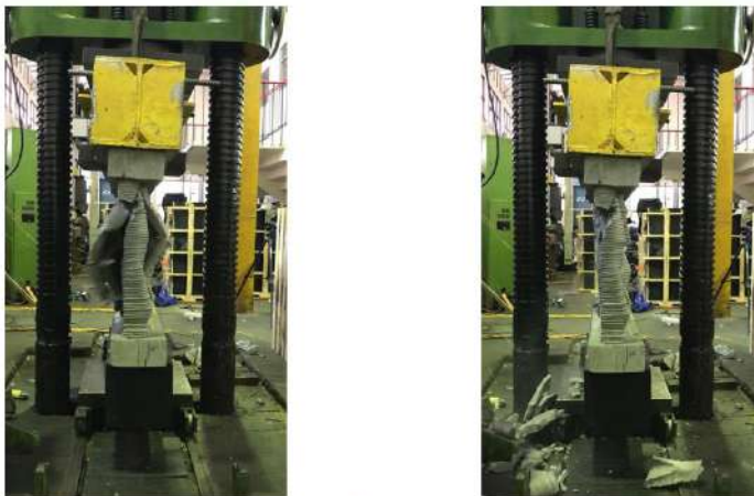
(a) at breaking of 3DP concrete shell (b) right after breaking of 3DP concrete shell
